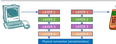
Data transfer occurs by breaking the file into small packets, adding each layer to the packet in order at the sending device, then decoding in reverse order at the receiving device before rebuilding the file.
