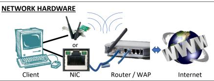
All clients need an NIC to connect to a ROUTER. This could be a wireless adapter or a network card. The Router in this simple connection can host multiple clients, but more advanced hardware is needed for bigger networks
