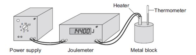
Before starting the experiment, the student reset the joulemeter to zero. The student switched the power supply on for exactly 10 minutes. During this time, the reading on the joulemeter increased to 14 400.
